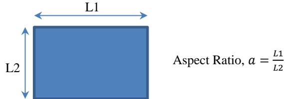
**Figure 1 – Aspect Ratio for a rectangular element**
