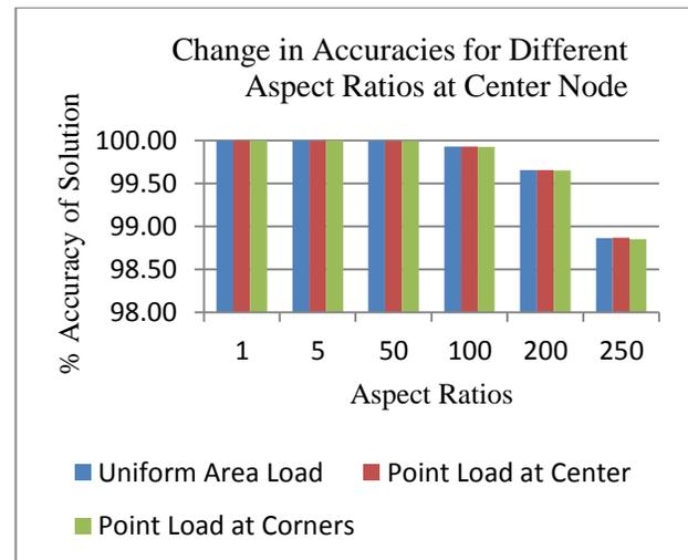
**Figures 3 – Graphs showing change in solution accuracy with aspect ratio at center and corner loads**
